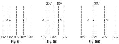
**Ans.** (c) The work done by a electrostatic force is given by  $W_{12} = q (V_2 - V_1)$ . Here initial and final potentials are same in all three cases and same charge is moved, so work done is same in all three cases.
