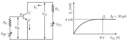
Given that the input impedance of the transistor is very small and  $V_{CC} = V_{BB} = 16$  V, also find the voltage gain and power gain of circuit making appropriate assumptions.
