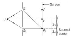
At  $P_2$  on the screen, there is a hole and behind  $P_2$  is a second 2-slit arrangement with slits  $S_3$ ,  $S_4$  and a second screen behind them.
