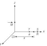
From figure, every point lies on the equatorial line of magnetic dipole. Magnetic field induction at a point distance x from the dipole is
