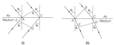
(i) Let *AB* represent the incident wavefront and *DE* represent the refracted wavefront. All points on a wavefront must be in same phase and in turn, must have the same optical path length.
