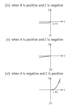
From these graphs of current - voltage characteristic shown in fig. (c) to (h) determine the arrangement of components between A, B, and C.
