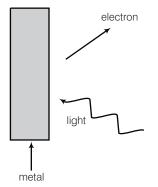
**Ans.** During photoelectric emission, the momentum of incident photon is transferred to the metal. At microscopic level, atoms of a metal absorb the photon and its momentum is transferred mainly to the nucleus and electrons.
