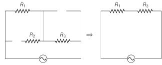
So, effective impedance =  $R_{eq} = R_1 + R_3$
