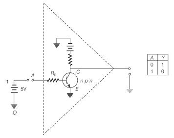
Here, the base *B* of the transistor is connected to the input *A* through a resistance  $R_b$  and the emitter *E* is earthed. The collector is connected to 5 V battery. The output Y is the voltage at *C* w.r.t. earth.
