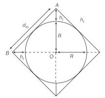
Suppose the height of transmitting antenna or receiving antenna in order to cover the entire surface of earth through communication is  $h_t$  and radius of earth is R. Then, maximum distance
