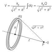
Considering -q charge at *P*, the potential energy is given by  $U = W = q \times \text{potential difference}$
