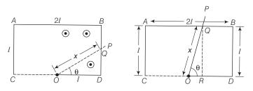
the rod *OP* will make contact with the side *BD*. Let the length *OQ* of the contact at sometime *t* such that  $0 < t < \frac{\pi}{4\omega}$  or  $0 < t < \frac{7}{8}$  be *x*. The flux through the area *ODQ* is
