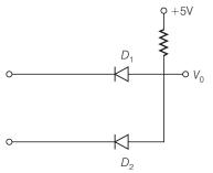
**Ans.** The circuit resemble AND gate. The boolean expression of this circuit is,  $V_0 = A.B.i.e.$ ,  $V_0$  equals A AND B. The truth table of this gate is as given below
