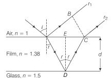
Refractive index of film = 1.38 and refractive index of glass = 1.5.  $\lambda = 5500 \text{ Å} .$
