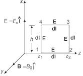
During the propagation of electromagnetic wave a long *z*-axis, let electric field vector (**E**) be along *x*-axis and magnetic field vector **B** along *y*-axis, *i.e.*,  $\mathbf{E} = E_0 \hat{\mathbf{i}}$  and  $\mathbf{B} = B_0 \hat{\mathbf{j}}$ .
