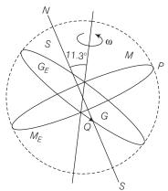
*P* is also on the magnetic equator, so the angle of dip = 0, because the value of angle of dip at equator is zero. *Q* is also on the magnetic equator, thus the angle of dip is zero. As earth tilted on its axis by  $11.3^{\circ}$ , thus the declination at *Q* is  $11.3^{\circ}$ .
