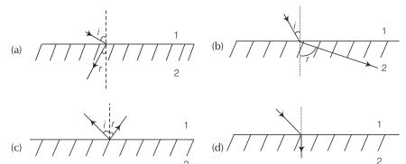
Ans. (a) The negative refractive index metamaterials are those in which incident ray from air (Medium 1) to them refract or bend differently to that of positive refractive index medium.
