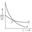
We know that  $\left(\frac{dN}{dt}\right) \propto \lambda_{A}$ , at any instant of time hence we can say that  $\lambda_{A} > \lambda_{B}$ . At point *P* shown in the diagram the two curve intersect.
