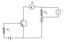
**Ans.** Consider the circuit in fig. (b) to find the change in reading As we know the formula for base current,  $I_B = \frac{V_{BB} - V_{BE}}{D}$
