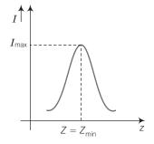
As frequency (v) increases, Z decreases and at certain value of frequency know as resonant frequency (v<sub>0</sub>), impedance Z is minimum that is  $Z_{min}=R$  current varies inversely with impedance and at  $Z_{min}$  current is maximum.
