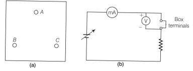
Three components namely, two germanium diodes and one resistor are connected across these three terminals in some arrangement.
